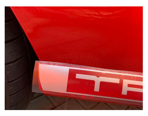
6. Peel off remaining backing, and apply remaining half of sticker
