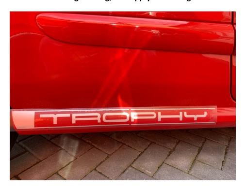
7. Gently rub over decal with a plastic card to help adhesion and remove any bubbles
